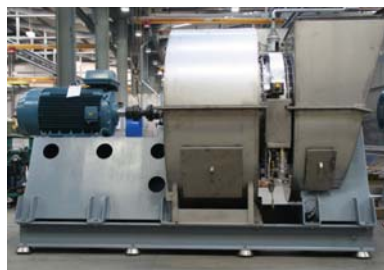
Halifax No 56 Backward curved fan designed to API 673, 2nd edition 2002.
